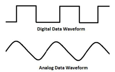
The main function of the modem is to convert digital signal into analog and vice versa. Modem is a combination of two devices – **modulator** and **demodulator**. The **modulator** converts digital data into analog data when the data is being sent by the computer. The **demodulator** converts analog data signals into digital data when it is being received by the computer.
