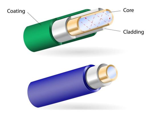
Optical fibre is rapidly replacing copper wires in telephone lines, internet communication and even cable TV connections because transmitted data can travel very long distances without
