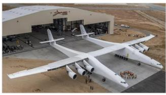
The aircraft is so big its wing span is longer than a football field, or about 1.5 times that of an Airbus A380. It hit a top speed of 304 kilometers per hour (189 mph) and reached an altitude of 17,000 feet, or 5,182 meters.
