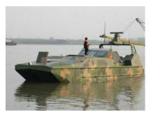
The drone ship has a maximum operation range of **1,200 km** and can be remotely controlled with the help of satellites.
