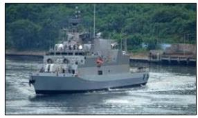
superstructure of carbon fibre composite material. INS Kiltan is also the first major warship to have undertaken sea trials of all major weapons and sensors as a pilot project.
