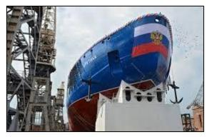
Russian ships delivering gas to Asia. Sibir is a double-draft design with a displacement of 33,500 tonnes and can carry out rescue work in ice conditions and ice-free waters.
