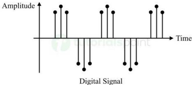
Digital signals are also called binary signals, as they use binary 0 or 1 to represent the state of a signal. Where, the binary 0 represents the off or low state of the signal, while the binary 1 represents the on or high state of the signal.
