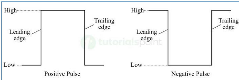
A pulse has two edges namely, a **leading edge** and a **trailing edge**.
