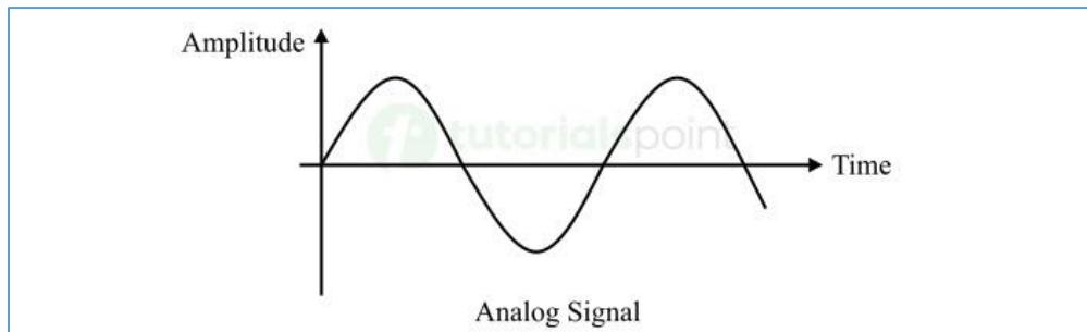
An important characteristic of analog signals is that they have a definite value at every instant of time, known as **instantaneous value of the signal**.
