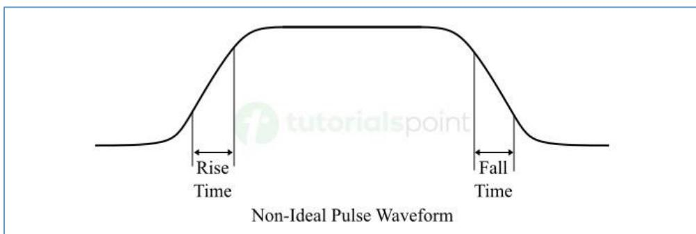
In the case of a non-ideal pulse waveform, the time taken by the pulse to go from low logic level to high logic level is called the **rise time**. The time taken by the pulse to go from the high logic level to the low logic level is called the **fall time**.
