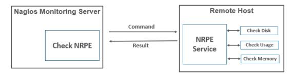
Let us see how to install and configure NRPE step by step on client machine which needs to be monitored.
