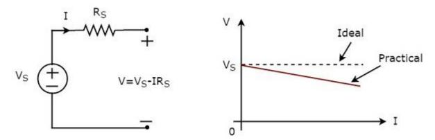
There is a deviation in the V-I characteristics of an independent practical voltage source from the V-I characteristics of an independent ideal voltage source. This is due to the voltage drop across the internal resistance ( $R_s$ ) of an independent practical voltage source.
