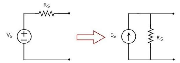
**Practical voltage source** consists of a voltage source  $(V_S)$  in series with a resistor  $(R_S)$ . This can be converted into a practical current source as shown in the figure. It consists of a current source  $(I_S)$  in parallel with a resistor  $(R_S)$ .
