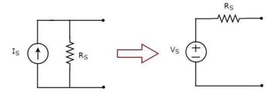
**Practical current source** consists of a current source ( $I_S$ ) in parallel with a resistor ( $R_S$ ). This can be converted into a practical voltage source as shown in the figure. It consists of a voltage source ( $V_S$ ) in series with a resistor ( $R_S$ ).
