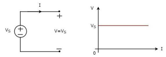
The **V-I characteristics** of an independent ideal voltage source is a constant line, which is always equal to the source voltage  $(V_s)$  irrespective of the current value (I). So, the internal resistance of an independent ideal voltage source is zero Ohms.
