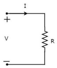
According to **Ohm's law**, the voltage across resistor is the product of current flowing through it and the resistance of that resistor. **Mathematically**, it can be represented as
