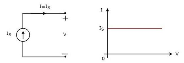
The **V-I characteristics** of an independent ideal current source is a constant line, which is always equal to the source current  $(I_S)$  irrespective of the voltage value (V). So, the internal resistance of an independent ideal current source is infinite ohms.
