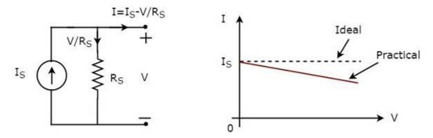
There is a deviation in the V-I characteristics of an independent practical current source from the V-I characteristics of an independent ideal current source. This is due to the amount of current flows through the internal shunt resistance ( $R_s$ ) of an independent practical current source.
