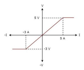
**Step 1:** Verifying the network element as **linear** or **non-linear**.
