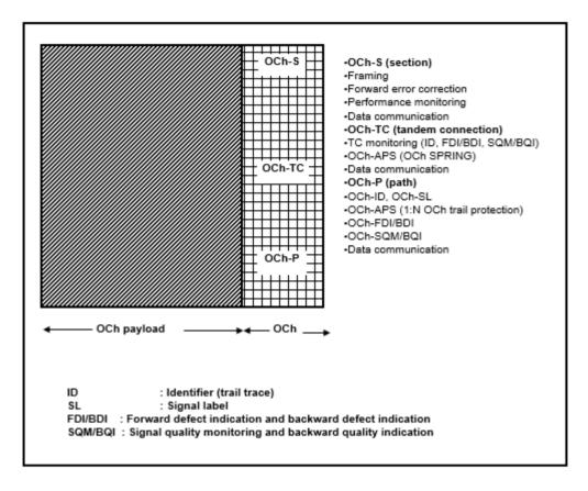
3R-regeneration (Reshaping, Retiming, and Regeneration) is provided by means of optical-to-electrical conversion and vice versa, and the digital wrapper proposal takes advantage of this. Would the picture change should all-optical 3R-regeneration becomes available? If all-optical regeneration is capable of adding overhead, the argument is unchanged; only the regenerator implementation would change.
