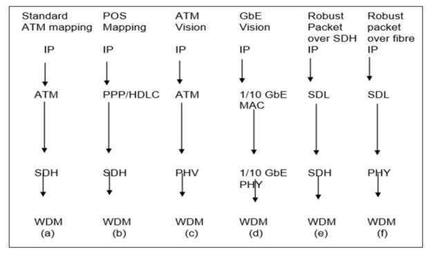
These different protocol stacks provide different functionality, in terms of bandwidth overhead, rate scalability, traffic management, and QOS. To state that any one particular mapping represents IP over WDM is extremely disingenuous.
