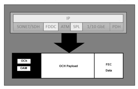
The notion of using a digital (or TDM) wrapper "around" the OCh client to support channel-associated OCh overhead has recently been proposed, and has in fact, been adopted as the basis for definition of the OCh. This scheme will take advantage of the need for OCh regeneration to add additional capacity to the OCh client. Of course, once we have a means of adding overhead to the OCh client signal digitally, it makes sense to use this to support all of the OCh-level OAM requirements.
