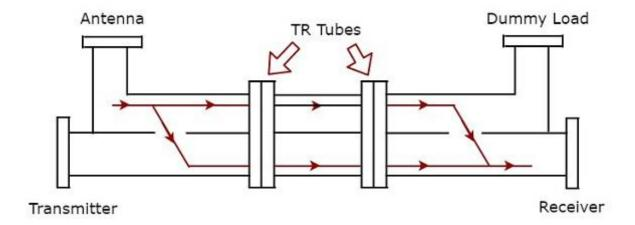
We know that Antenna receives the signal during reception time. The signal which is received by the Antenna has to reach the receiver. The **solid lines with arrow marks** shown in the above figure represent how the signal is reaching the receiver from Antenna. In this case, Dual TR tubes pass the signal from the first section of waveguide to the next section of waveguide.
