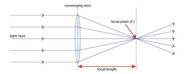
The **ray diagram** represents the focal point and the focal length from the source to the Lens. The parallel rays obtained are also called collimated rays.
