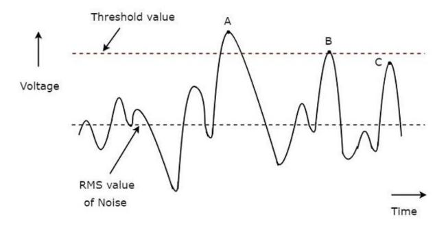
A **typical waveform** of the Radar receiver is shown in the above figure. The x-axis and y-axis represent time and voltage respectively. The rms value of noise and threshold value are indicated with dotted lines in the above figure.
