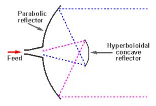
The above figure shows the working model of the cassegrain feed.
