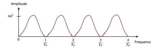
The frequency response characteristics of both double delay line canceller and the cascaded combination of two delay line cancellers are the same. The **advantage** of time domain delay line canceller is that it can be operated for all frequency ranges.
