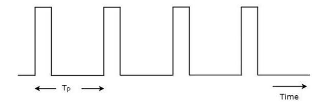
As shown in the figure, Radar transmits a periodic signal. It is having a series of narrow rectangular shaped pulses. The time interval between the successive clock pulses is called **pulse repetition time**,  $T_P$ .
