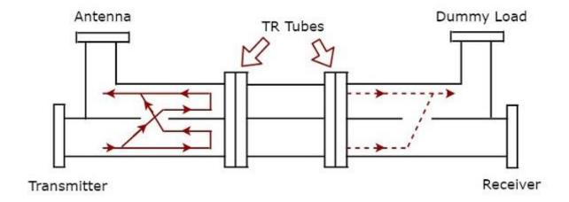
The signal, which is produced by the transmitter has to reach the Antenna for the Antenna to transmit that signal during transmission time. The **solid lines with arrow marks** shown in the above figure represent how the signal reaches Antenna from transmitter.
