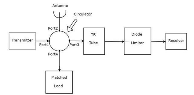
The following figure shows the **block diagram** of circulator as Duplexer:
