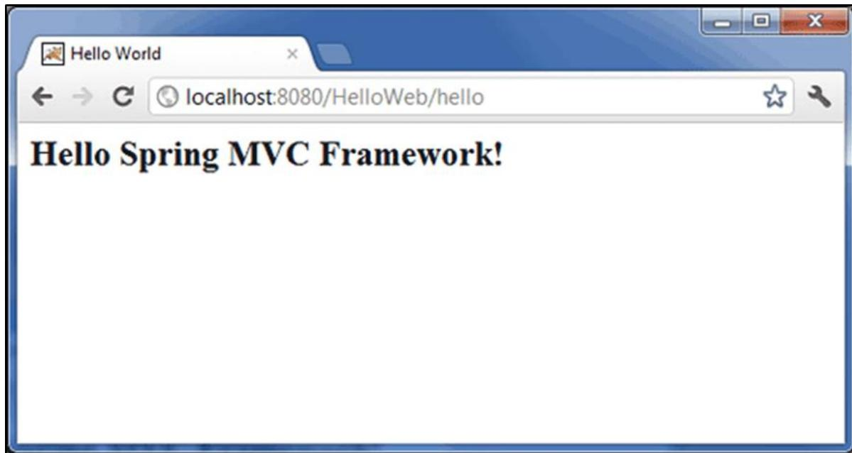
You should note that in the given URL, **HelloWeb** is the application name and **hello** is the virtual subfolder, which we have mentioned in our controller using `@RequestMapping("/hello")`. You can use direct root while mapping your URL using `@RequestMapping("/")`, in this case you can access the same page using short URL **http://localhost:8080/HelloWeb/**, but it is advised to have different functionalities under different folders.
